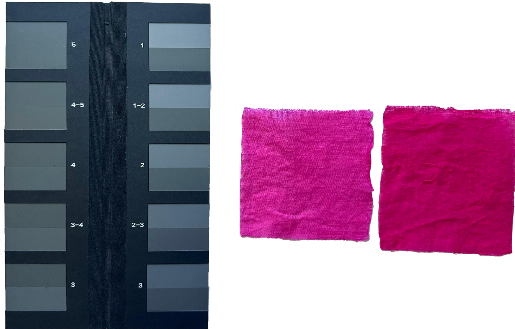
Figures 172 – 176. RR195 light-fastness test, including ISO Grey Scale comparison (before/after light) and full experimental workflow. All photographs by author.
