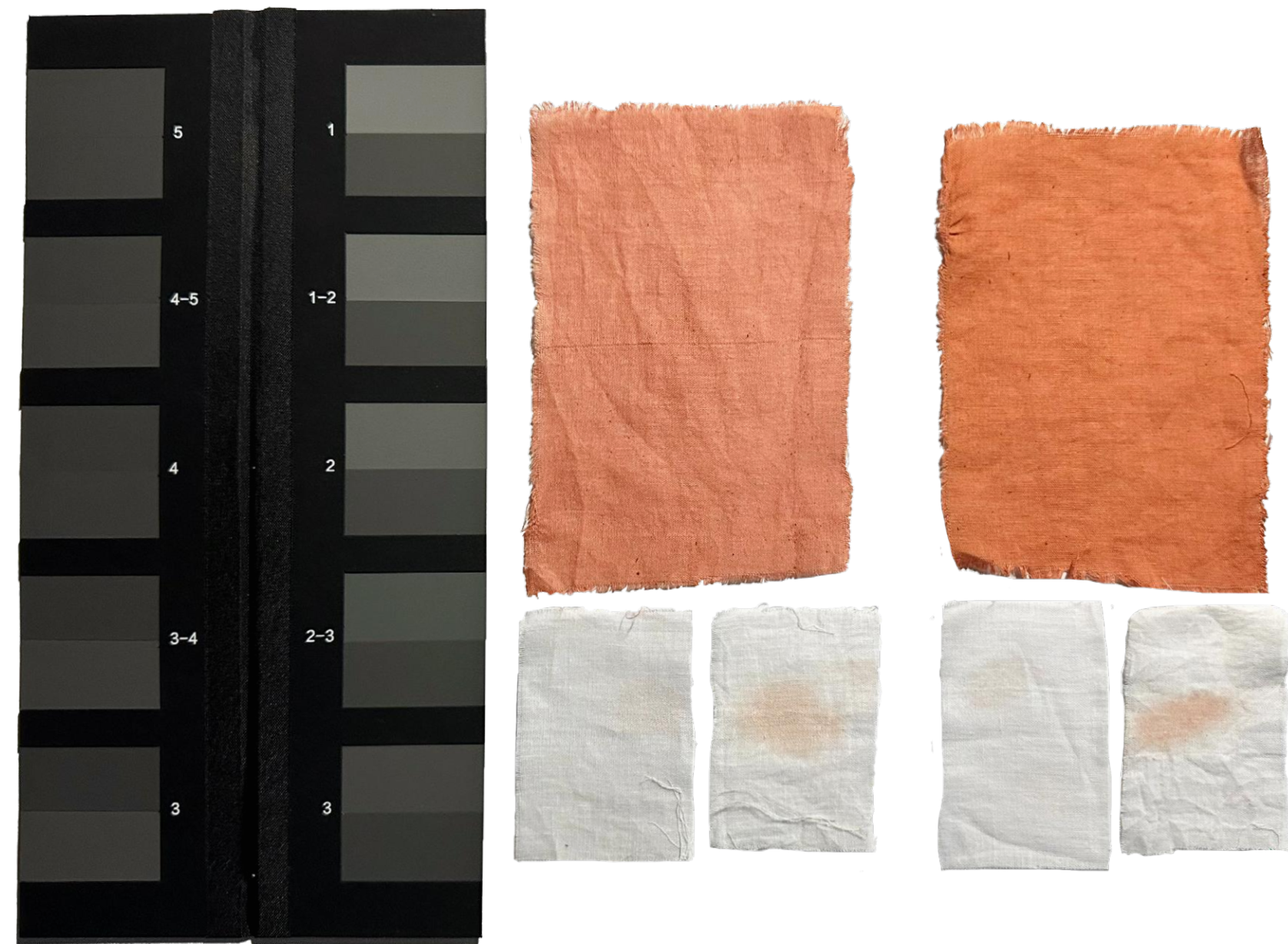
Figures 130 – 138. India Madder rubbing-fastness test, including ISO Grey Scale comparison (before/after rubbing) and full experimental workflow. All photographs by author.
