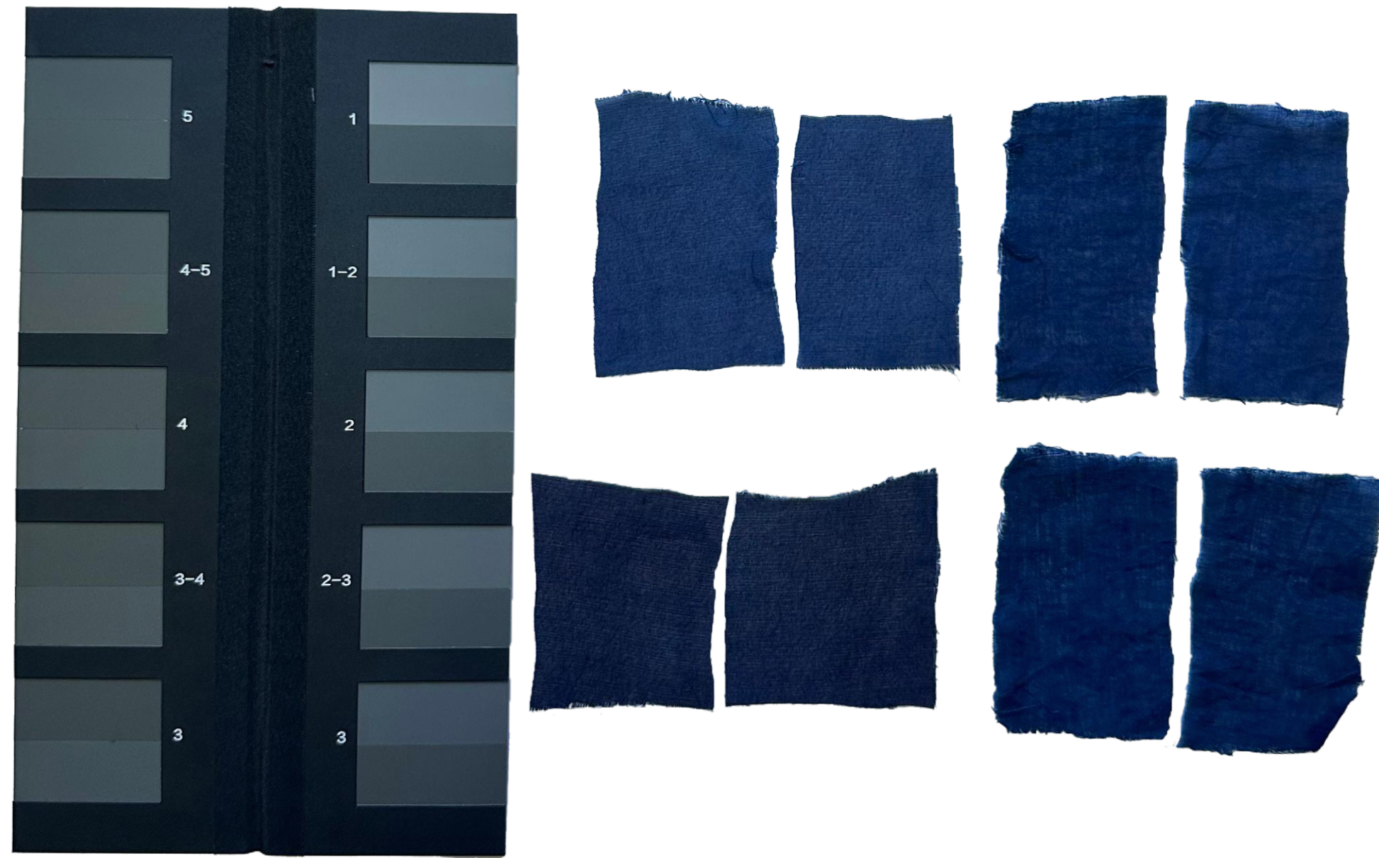
Figures 177 – 182. Indigo perspiration-fastness test, including ISO Grey Scale comparison (before/after perspiration) and full experimental workflow. All photographs by author.
