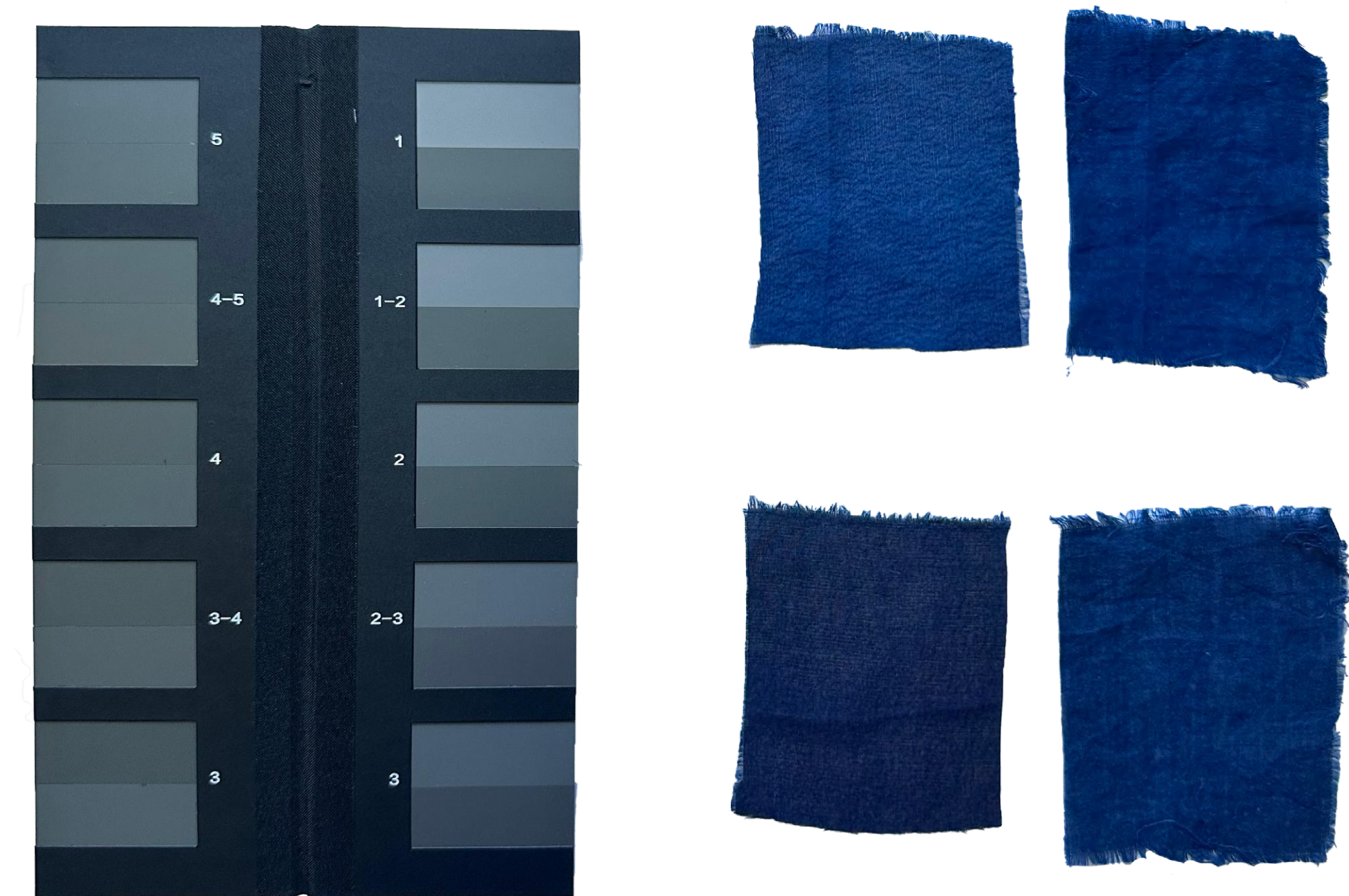
Figures 149 - 154. Indigo light-fastness test, including ISO Grey Scale comparison (before/after light) and full experimental workflow. All photographs by author.
