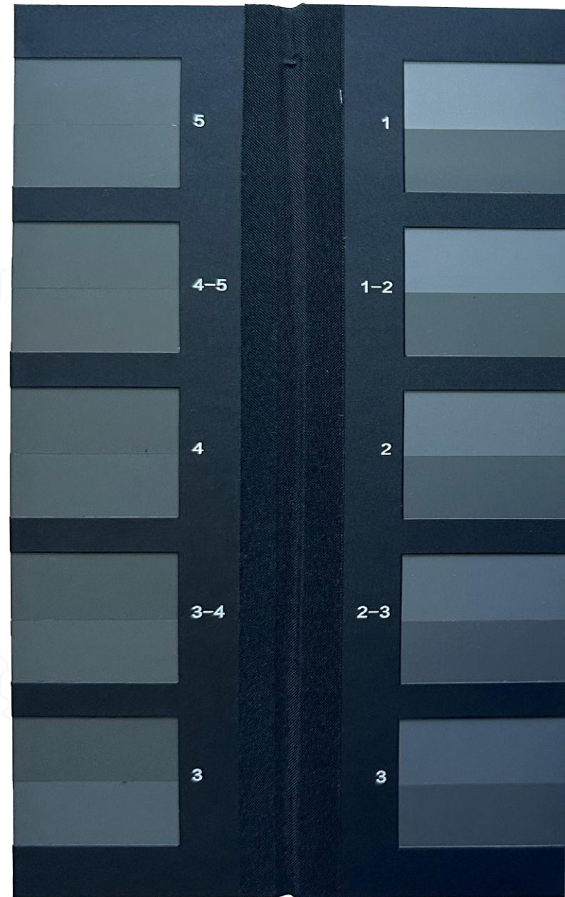
Figures 161 – 166. India Madder light-fastness test, including ISO Grey Scale comparison (before/after light) and full experimental workflow. All photographs by author.
