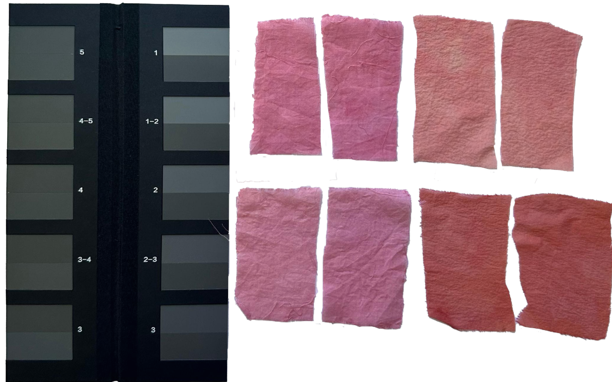
Figures 183 – 187. China Madder perspiration-fastness test, including ISO Grey Scale comparison (before/after perspiration) and full experimental workflow. All photographs by author.
