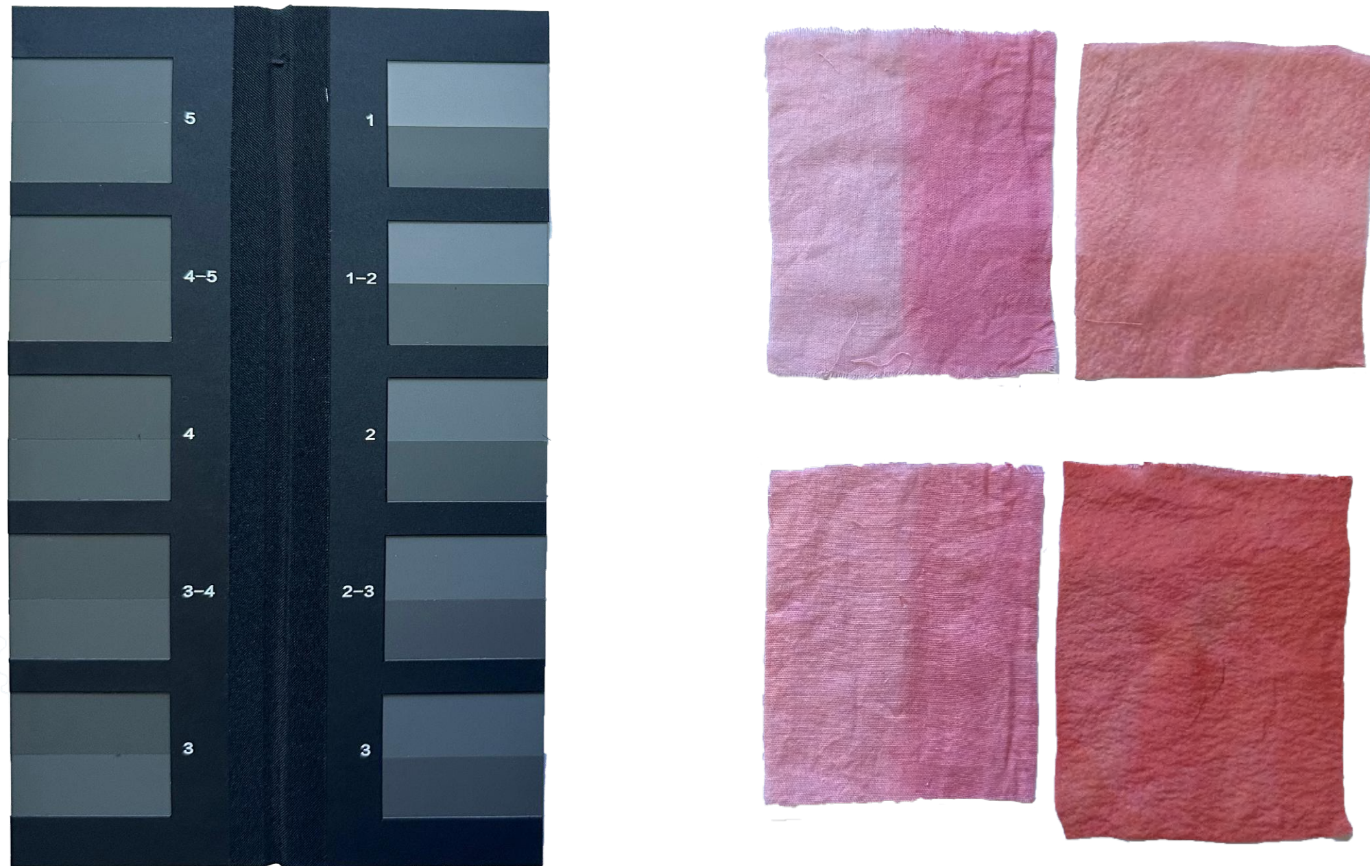
Figures 155 – 160. China Madder light-fastness test, including ISO Grey Scale comparison (before/after light) and full experimental workflow. All photographs by author.
