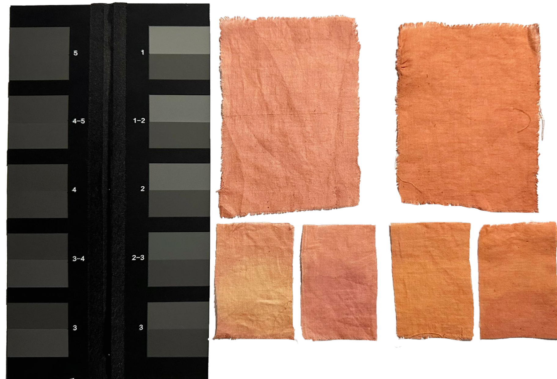
Figures 188 – 190. India Madder perspiration-fastness test, including ISO Grey Scale comparison (before/after perspiration) and full experimental workflow. All photographs by author.
