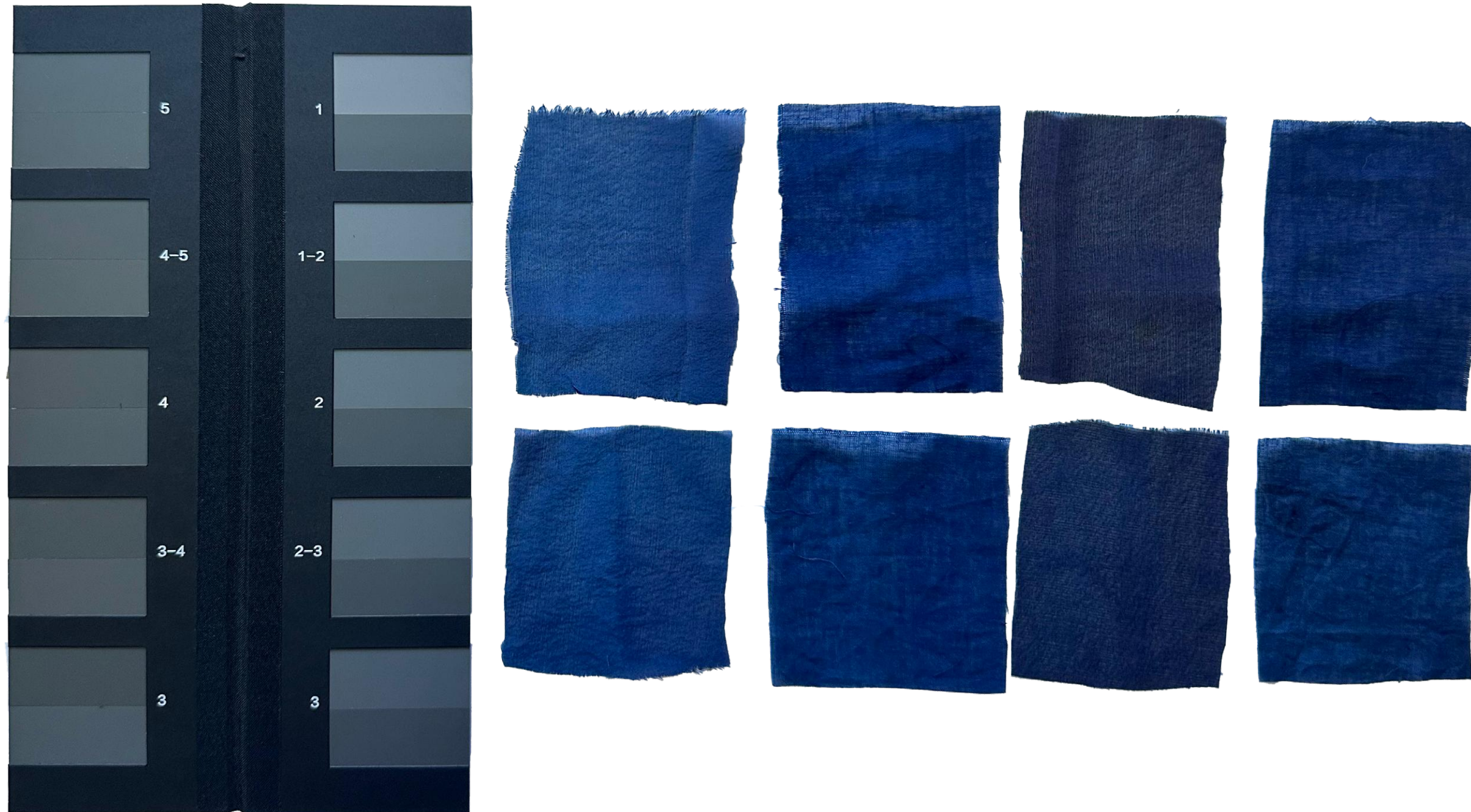
Figures 67 – 72. Indigo wash-fastness test, including ISO Grey Scale comparison (before/after wash) and full experimental workflow. All photographs by author.
