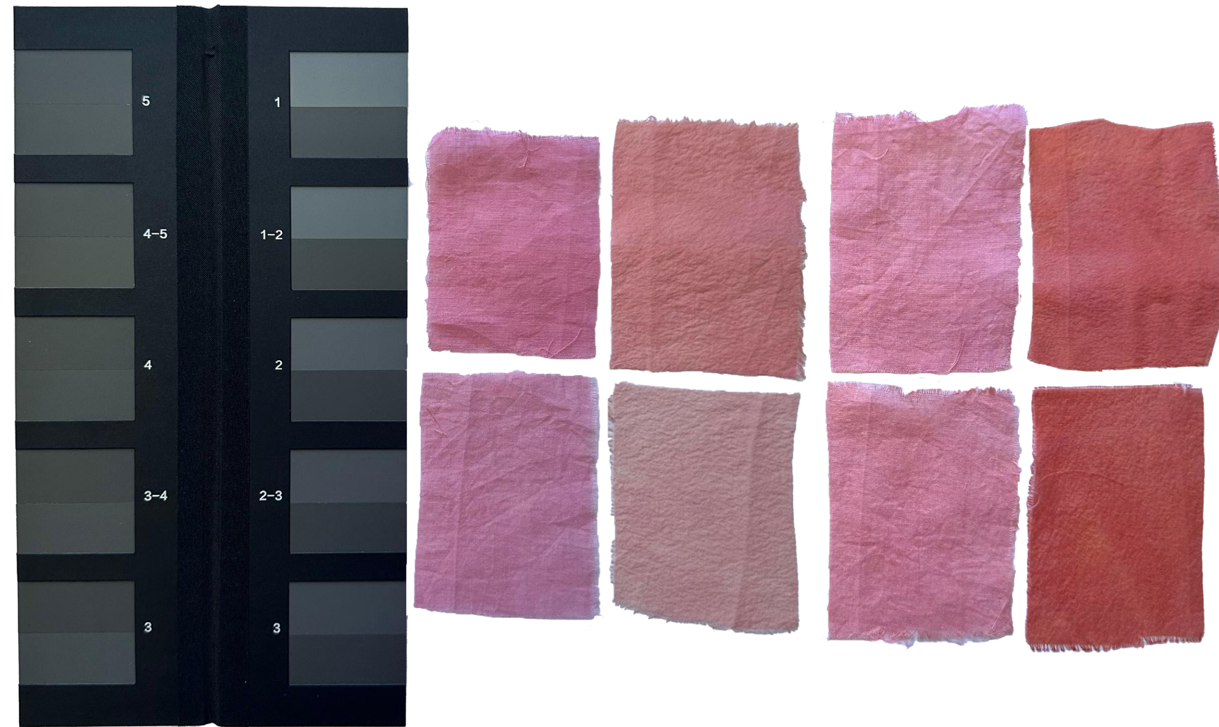
Figures 73 – 78. China Madder wash-fastness test, including ISO Grey Scale comparison (before/after wash) and full experimental workflow. All photographs by author.
