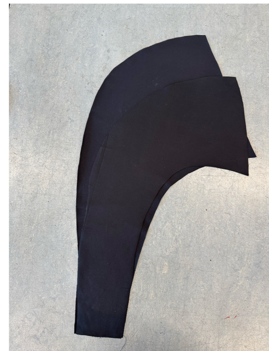
Figure 8. Basic two-piece sleeve pattern. Front sleeve panel (left), back sleeve panel (right).
