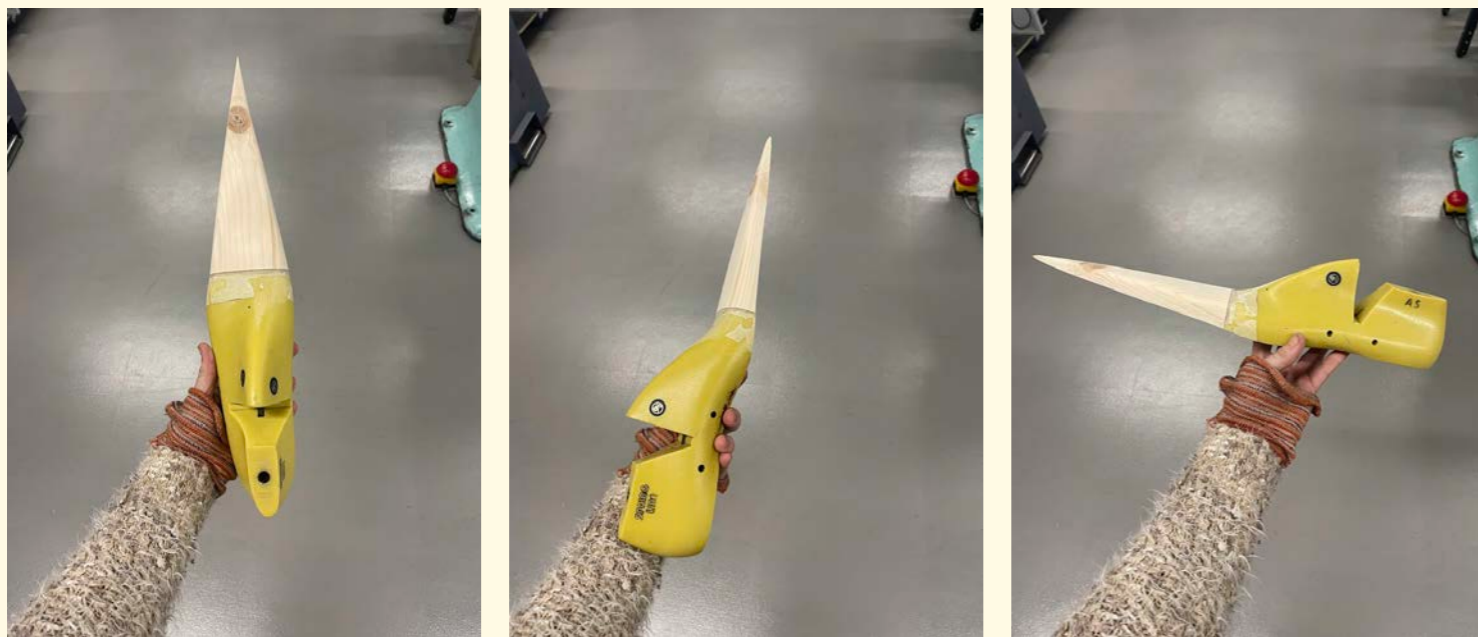
Figures show the original last prototype with minimal toe spring and a plastic donor last, causing problems boning to the wooden extension.
