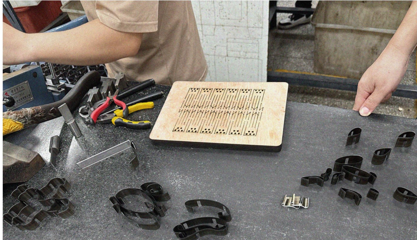
Fig. 33, Below, Tiancheng Meng, Cutting-die manufacturing process - assembling blades, 2025
