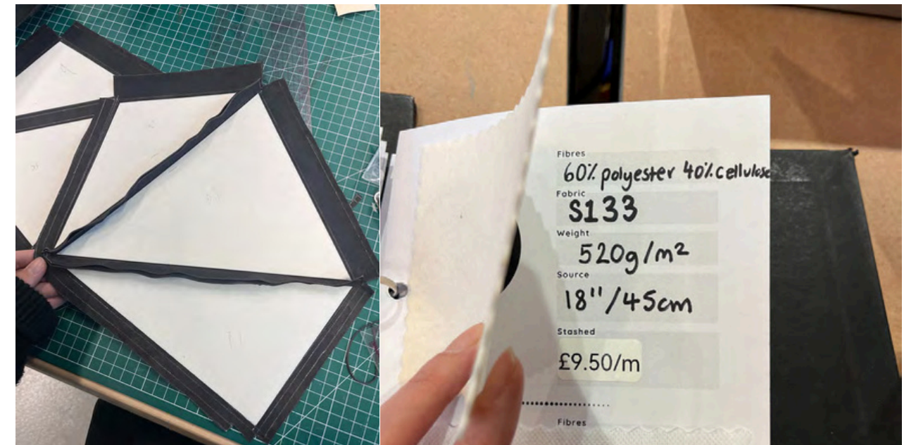
Tests on the adhesion of leather to different hardness backing fabrics and different number of layering repetitions
