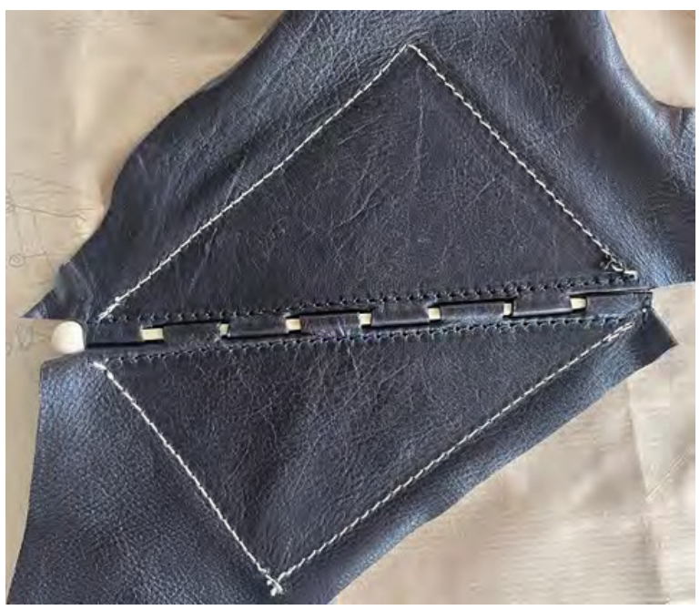
Figure 15. Sample of connection made with leather strips and wooden sticks.
