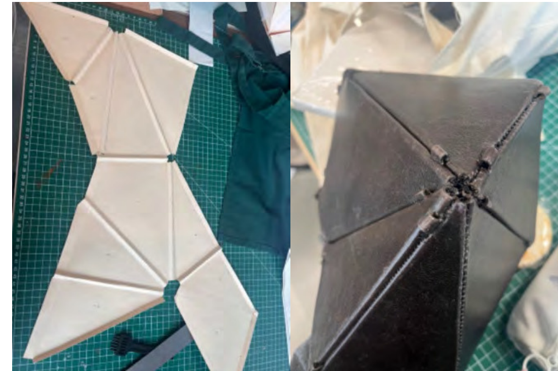
Early pattern-cutting sample showing geometric distortion at corner joints.
