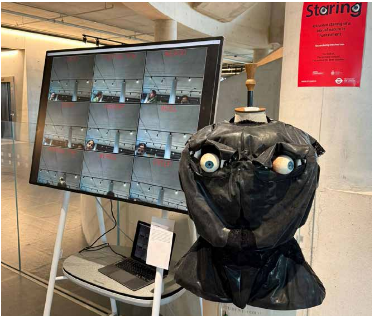
Figure 5: First iteration of the ‘Monstrous Vision’ garment. The garment features a hidden face-detection camera and mechanical eyes that would open once a face was detected.
