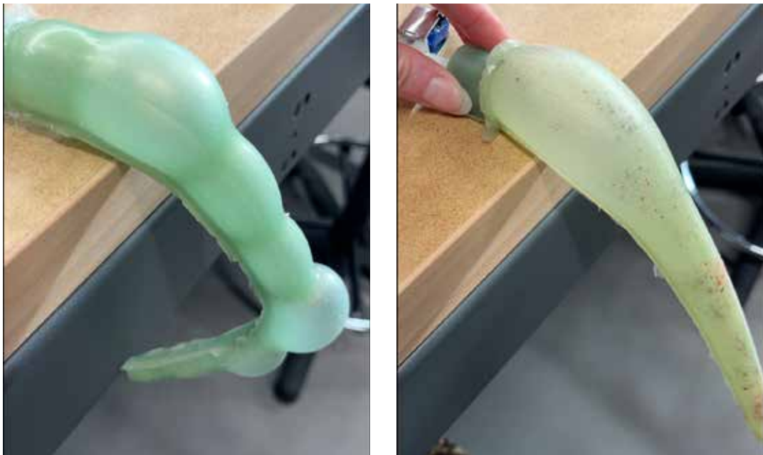
Figure 14: Iterations of the inflatable tentacle; one ribbed that bends well and one without ribbing that grows in size. I combined these two styles to produce the final tentacles.
