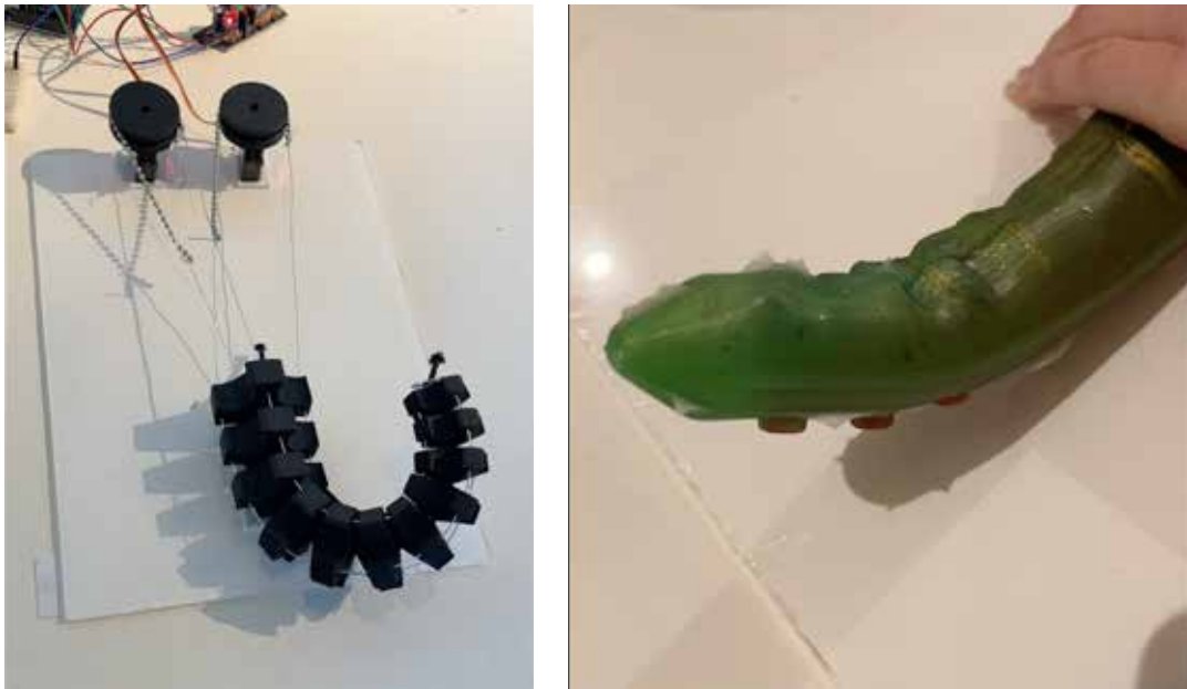
Figure 13: An early iteration of the motorised tentacle and the motorised tentacle with its silicone skin. The skin features imperfections from the casting process.
