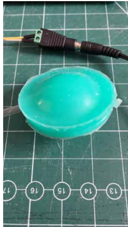
Figure 17: Large and small pocket inflation tests. The larger pieces were unsuccessful, but the small tests inflated well.
