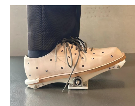
Prototype 4 Mount the shoes onto a seesaw-like platform device.
