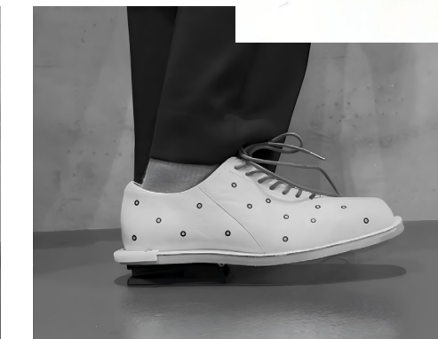
Prototype 3 The mechanical device on the left shoe is installed at the heel, while the one on the right shoe is installed at the forefoot.
