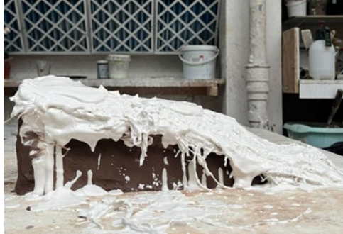
Fig.53 First plaster mold-making process
