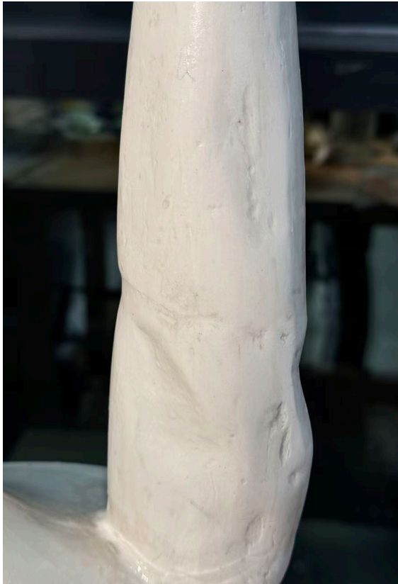
There are many small pits on the surface of the arm
