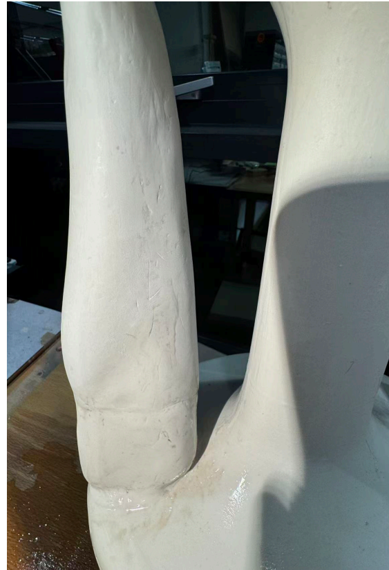
There are many small pits on the surface of the arm
