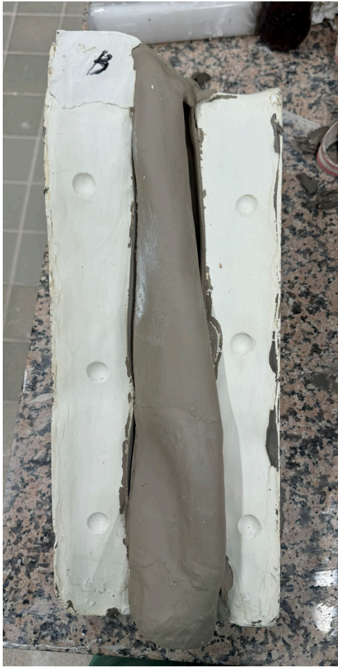
The clay arm using Arm B's plaster model was pulled in two.
