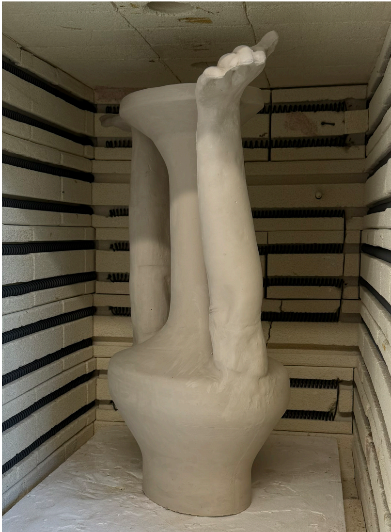
The slip casting piece retains air pockets. After two days of rapid drying in the kiln, no cracking occurred!
