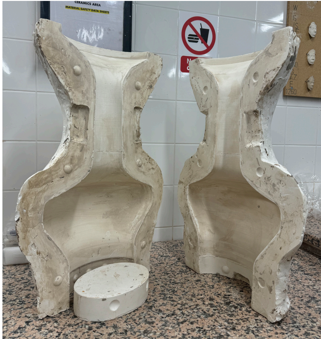
The three parts of the plaster model that makes up the vessel
