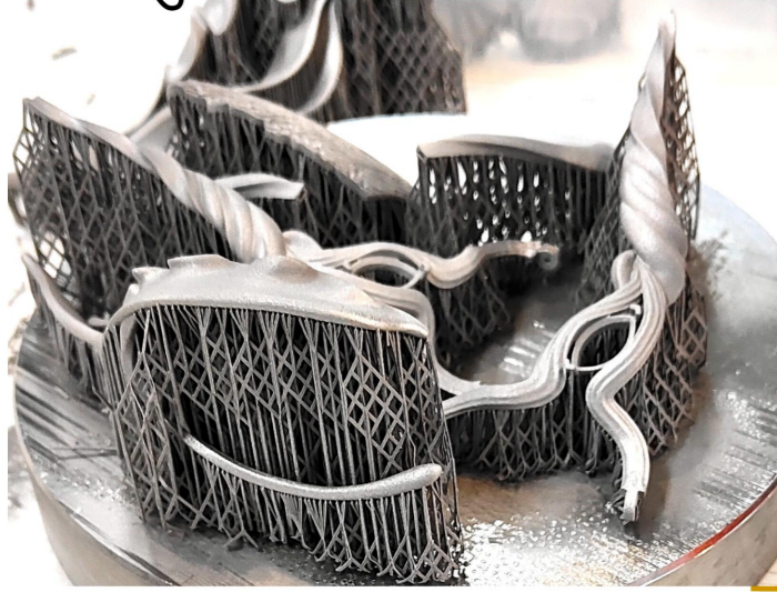
Sintering titanium metal powder
