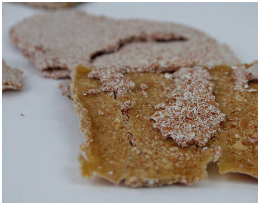
Gelatin 1 Brittle texture, not as stable, partially separated ingredients.
