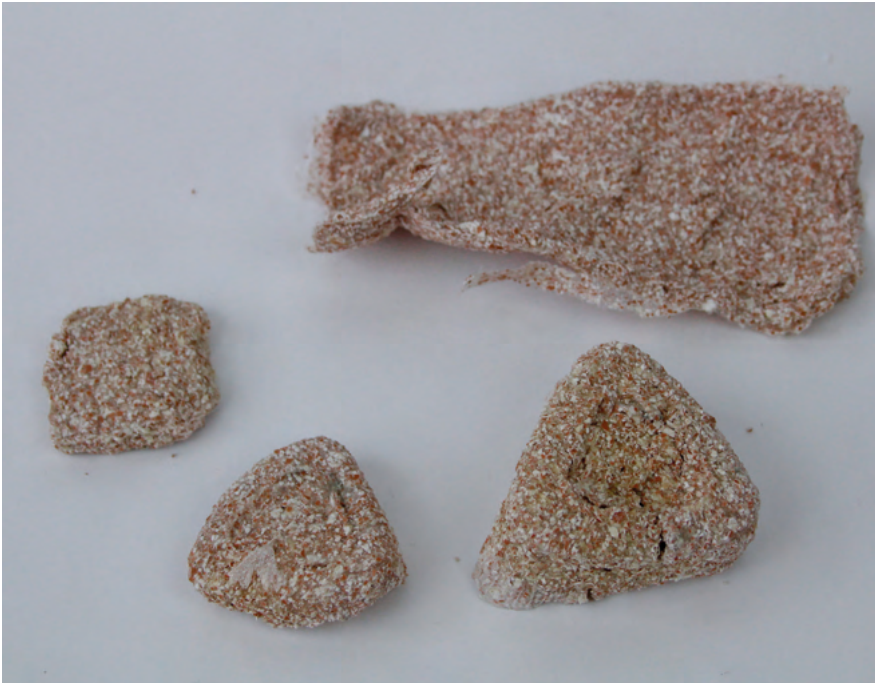
Starch 1 Dense and stable, develops mold while drying on bigger pieces.
