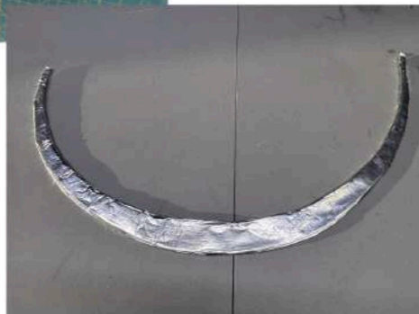
Lacked structural support → shifted to metal bar construction
