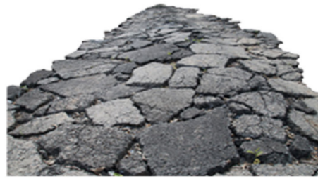
Asphalt chunks are mixed into an asphalt recycler along with water and additives
