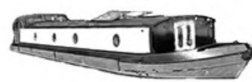
WIDE BEAM NARROW BOATS width range between 3.05 to 3.66 meters length varies and can extend upto 21.34 meters
