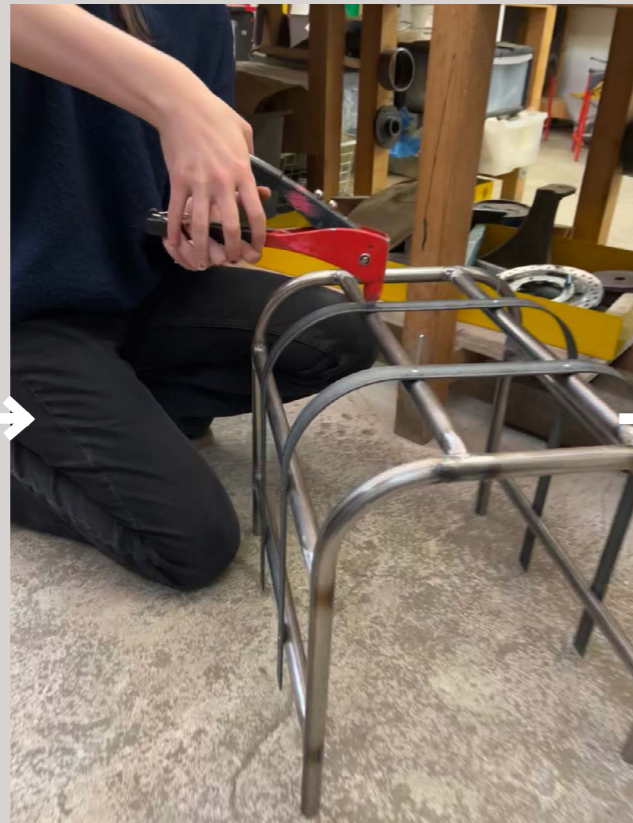
Connecting the steel using rivits.
