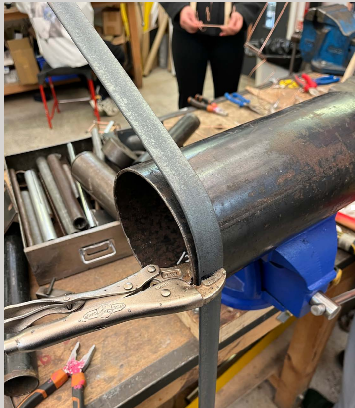
Bending flatbar to go over metal structure.
