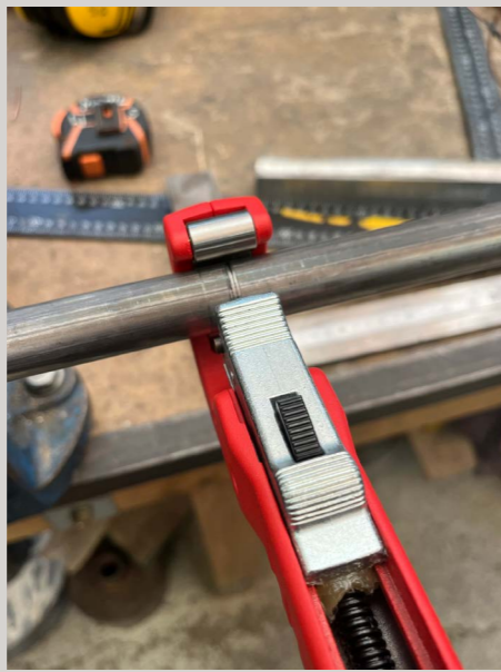
Cutting and bending steel pipe.
