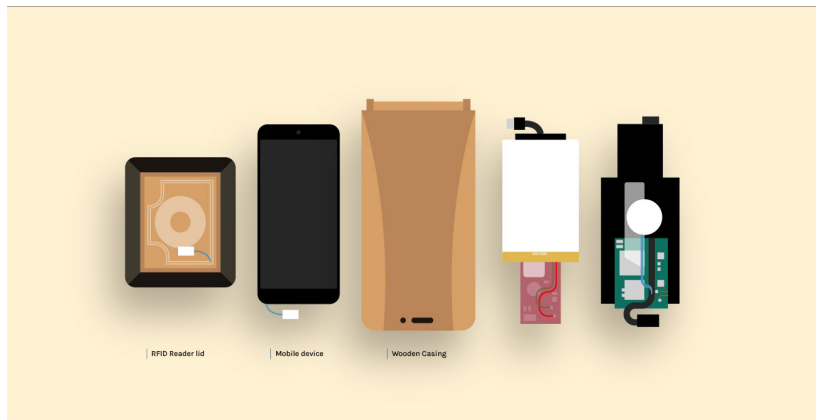
Figure 9. Devices inside wooden casing
