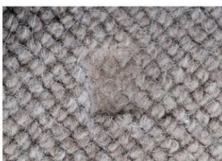
Carpet indentation The desk is placed in one place for a long time and the legs of the desk leave an indentation in the carpet.
