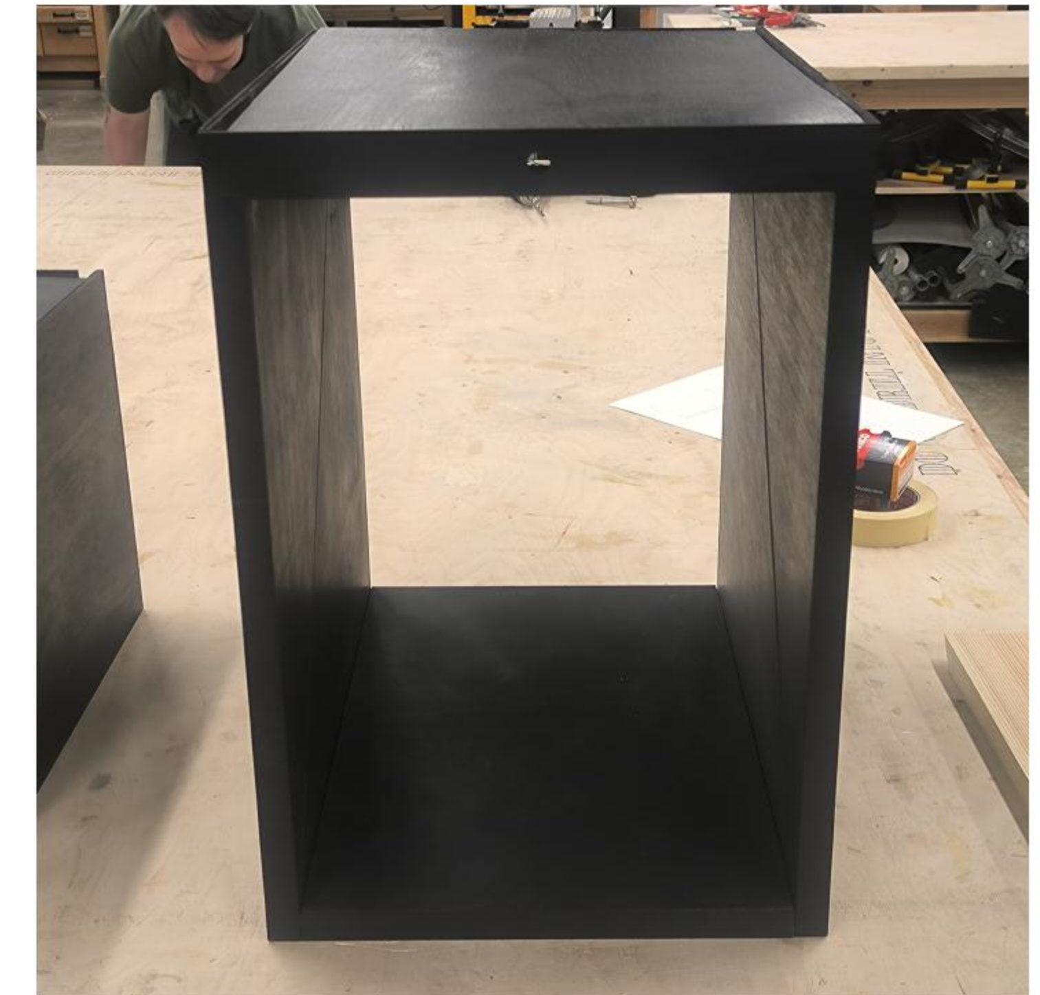
Finally, wax was applied in three layers, with the surface polished after each application.
