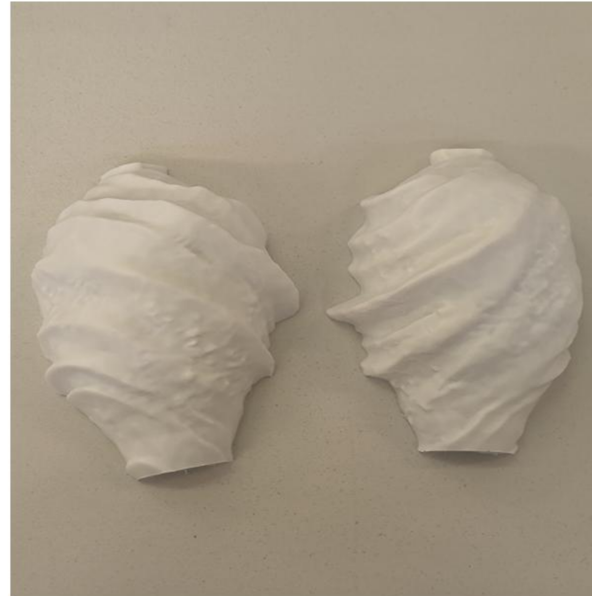
To facilitate the removal of internal supports, the model was divided into two parts for printing.
