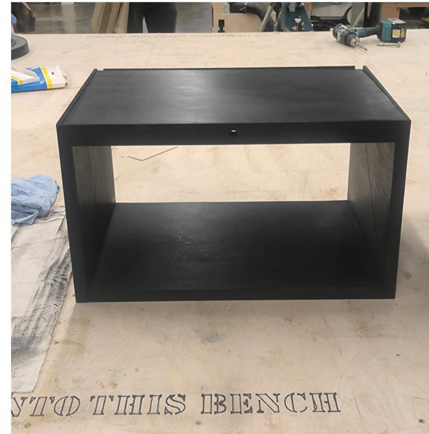
Finally, wax was applied in three layers, with the surface polished after each application.
