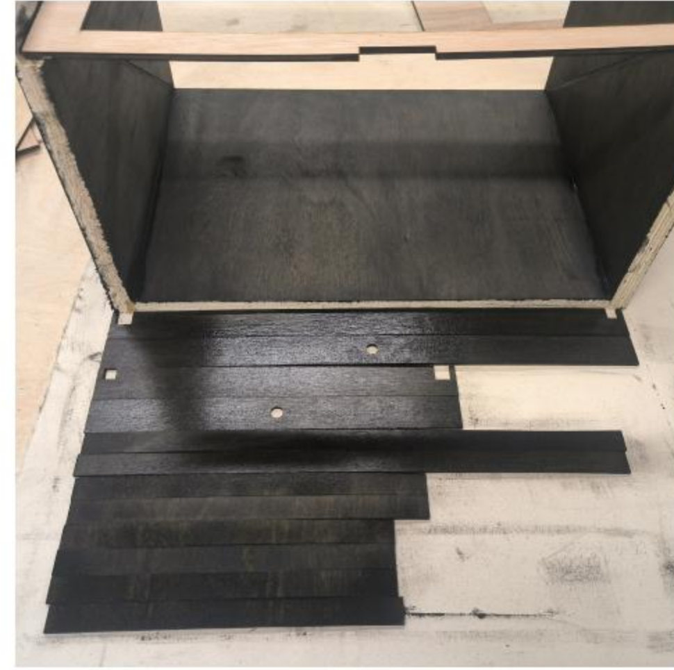
Since recycled wood was used, I first sanded off the surface's old adhesives and paint. Then, I applied wood stain to recolor the material.
