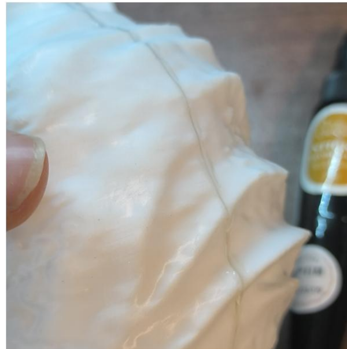
Assemble the model, then use UV glue to bond the pieces together and fill in the seams.
