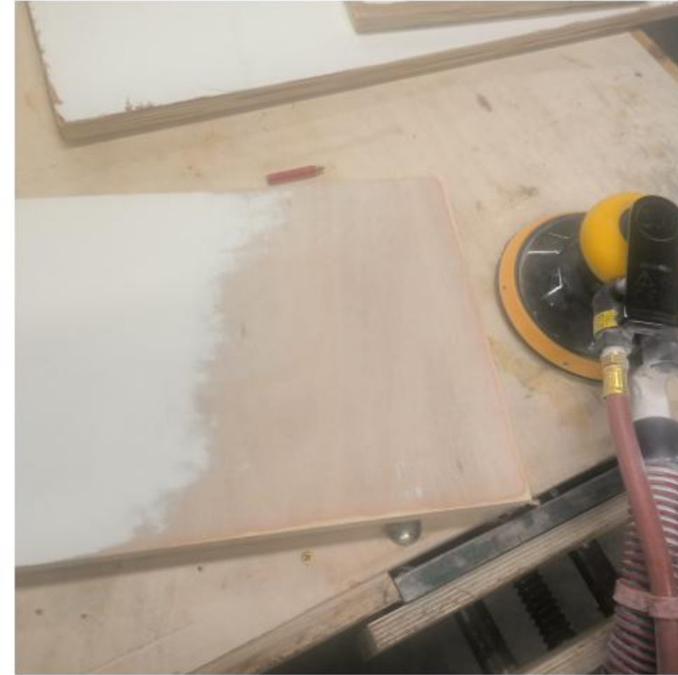
Since recycled wood was used, I first sanded off the surface's old adhesives and paint. Then, I applied wood stain to recolor the material.
