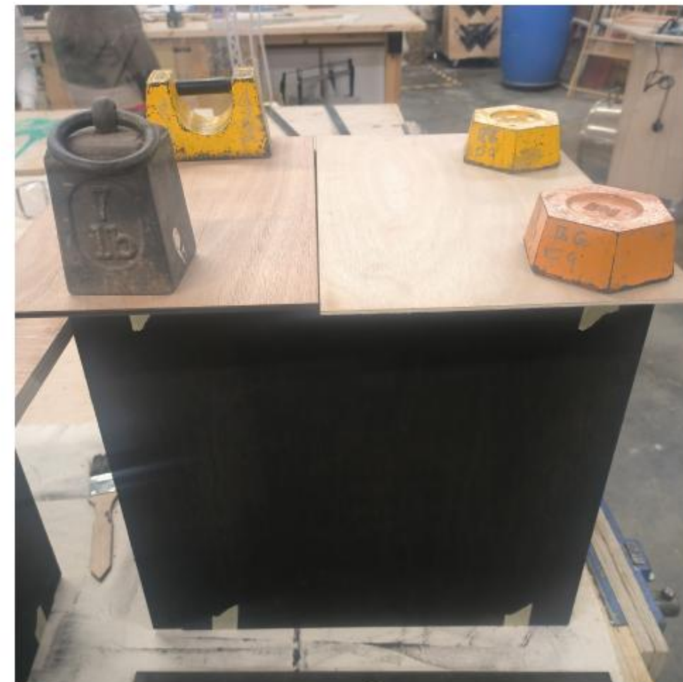
Next, the wooden panels were bonded together, with clamps used to provide additional reinforcement during the process.
