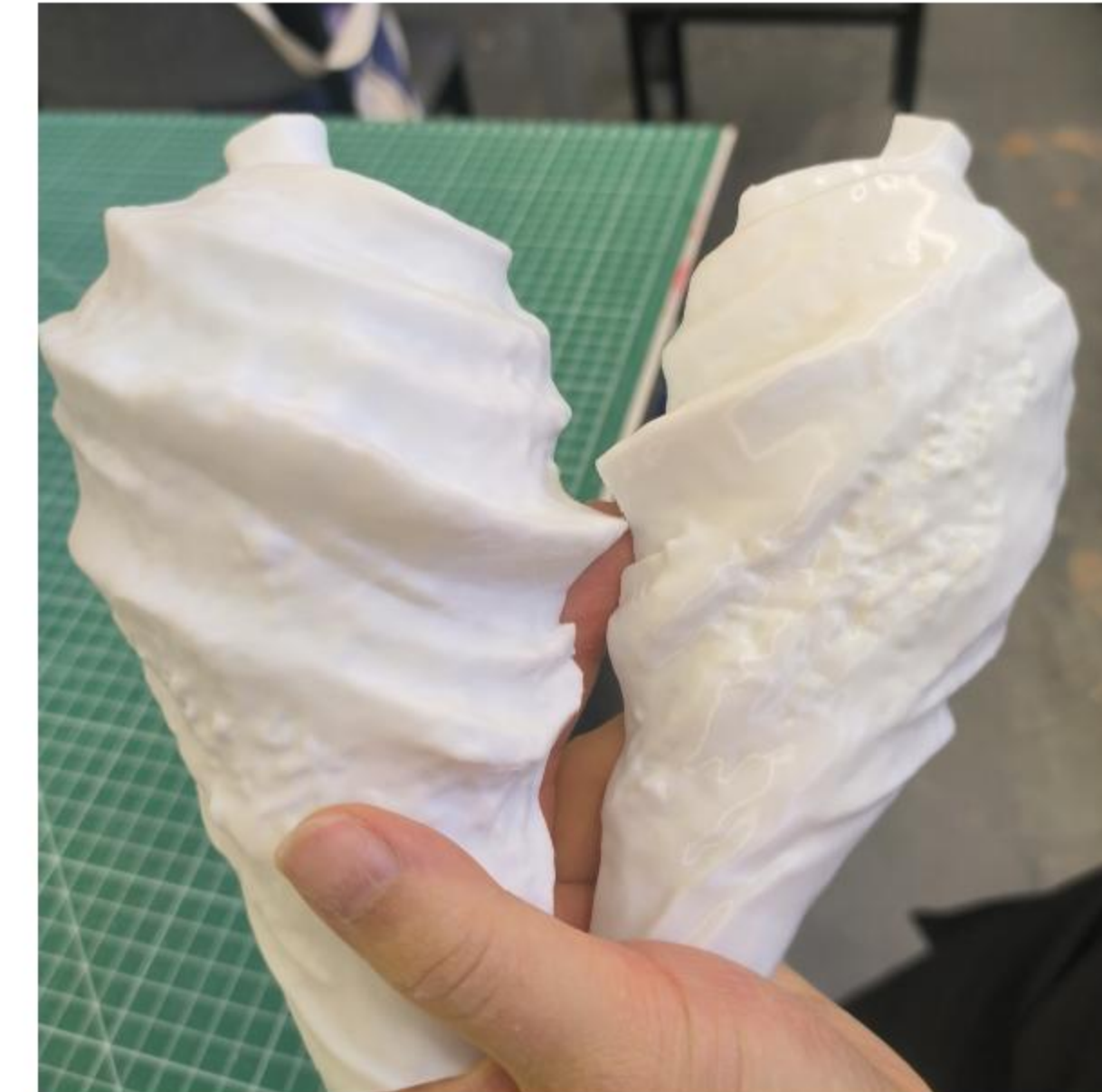
Sanding to remove layer lines (comparison of before and after sanding shown on the left and right).
