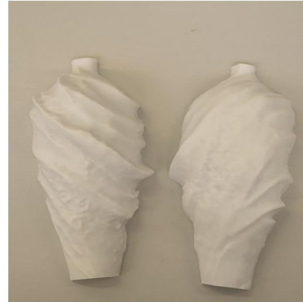
To facilitate the removal of internal supports, the model was divided into two parts for printing.
