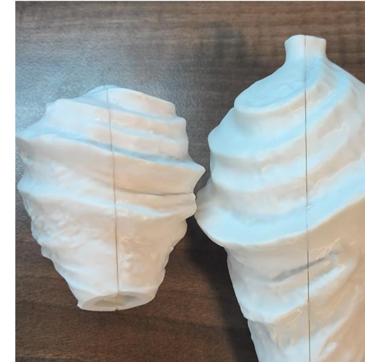
Sanding to remove layer lines (comparison of before and after sanding shown on the left and right).
