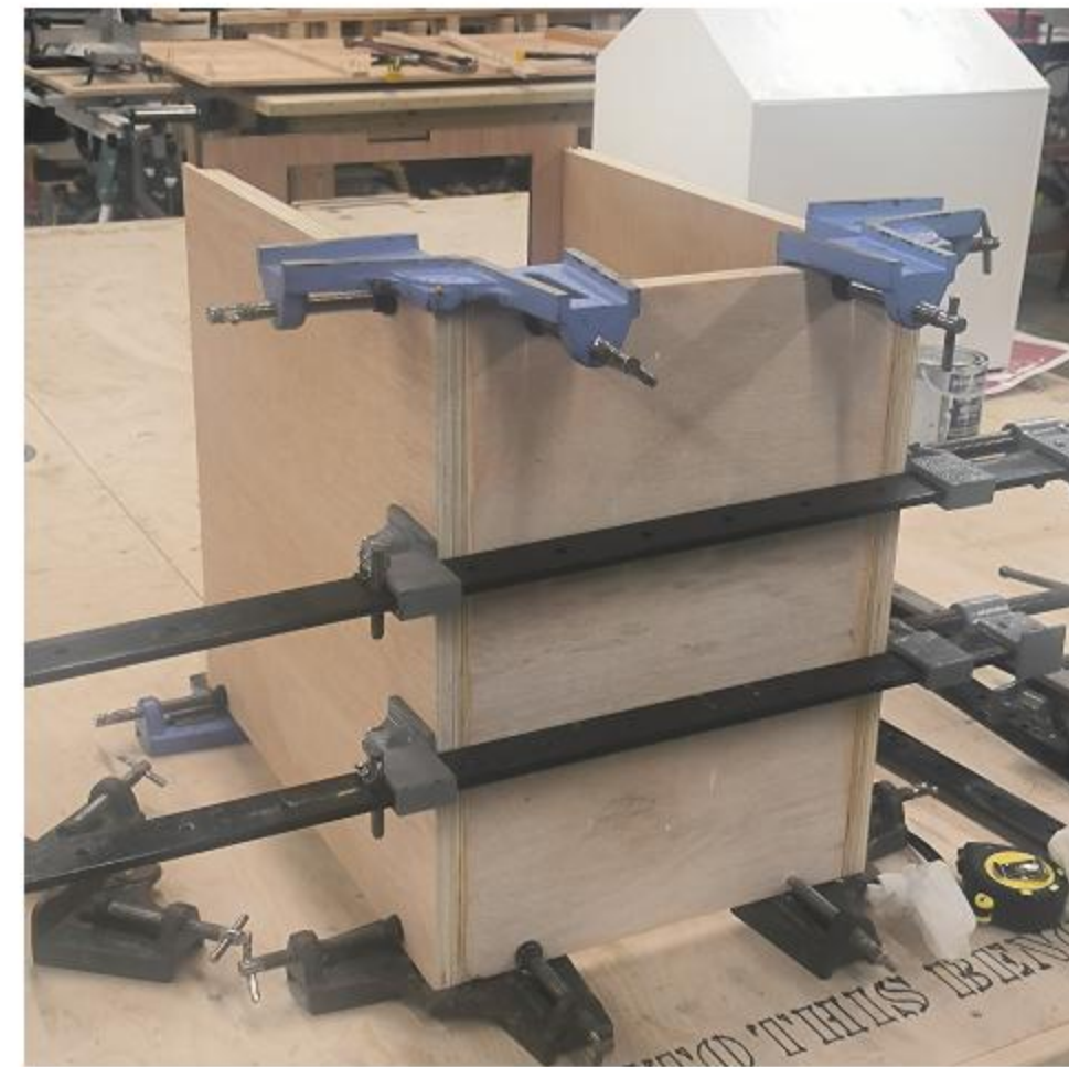
Next, the wooden panels were bonded together, with clamps used to provide additional reinforcement during the process.
